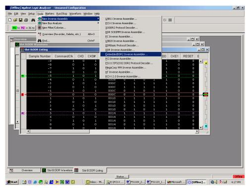
After the decoder has loaded, select Preferences if required, from the overview screen and set the preferences to their correct value in order to decode the trace properly. This is a general requirement, some decoders do not have preferences, if this is the case then no preference setting is necessary.
